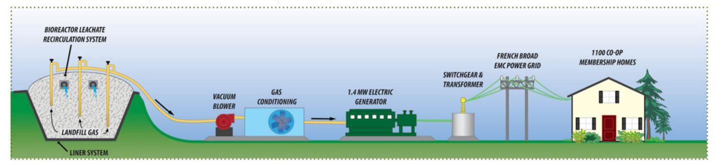
The landfill Gas to Energy Project began in 2010 with the installation of gas collection wells at the landfill. These wells tap the methane gas that is produced as trash decomposes in the landfill. Instead of releasing this powerful greenhouse gas into the air, which can negatively affect air quality, the wells capture it and divert it to run a generator. The generator creates electricity from this gas reducing the demand for coal or natural gas which are both non-renewable resources.
