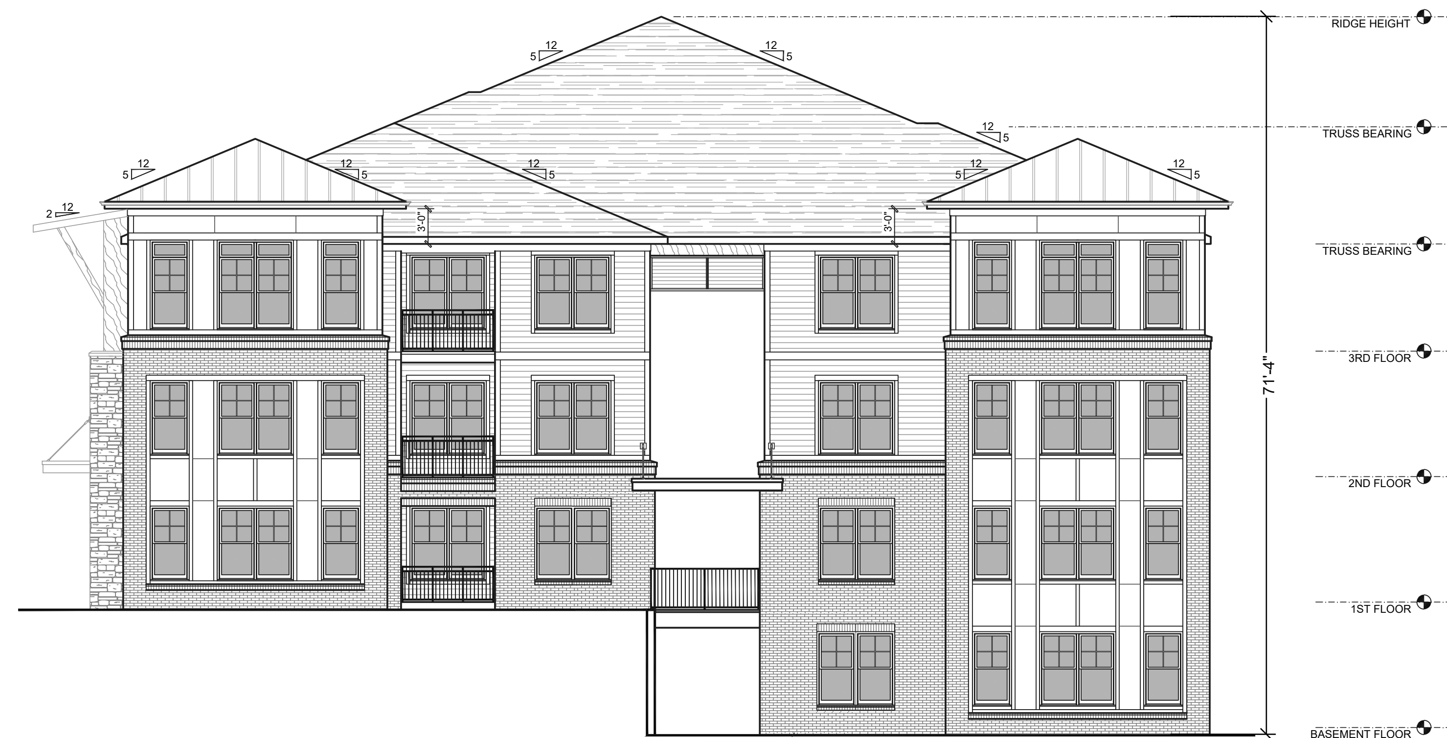
BUILDING TYPE 1 - SIDE ELEVATION
