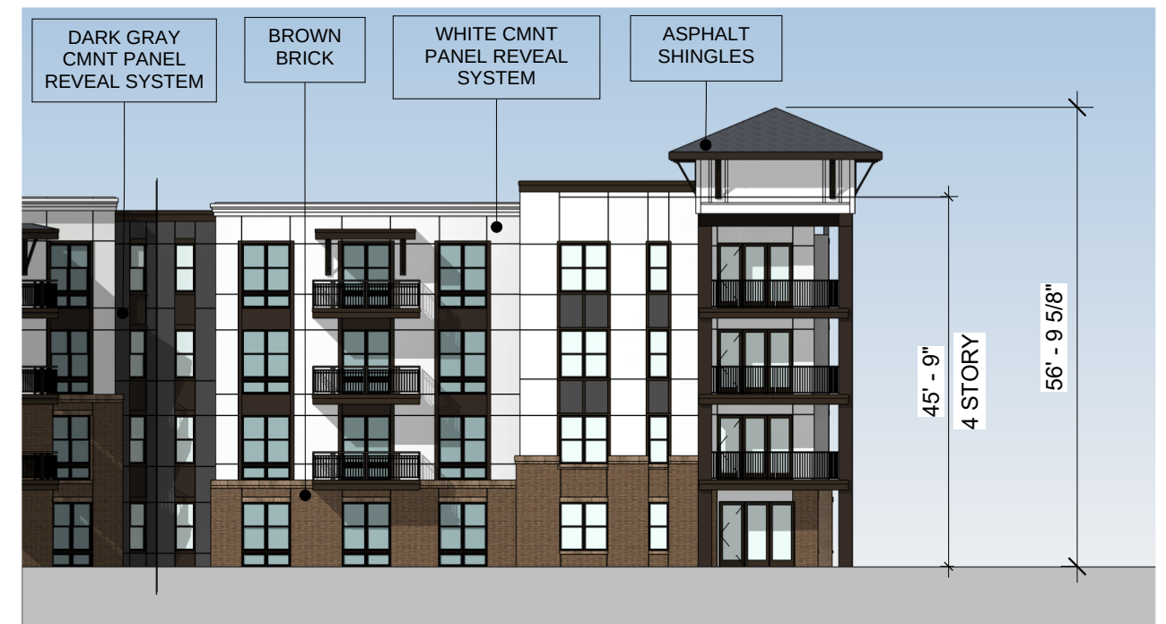
BUILDING 100 - ELEVATION PART B
