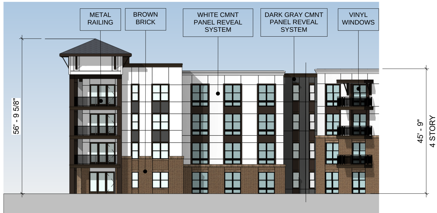
BUILDING 100 - ELEVATION PART A
