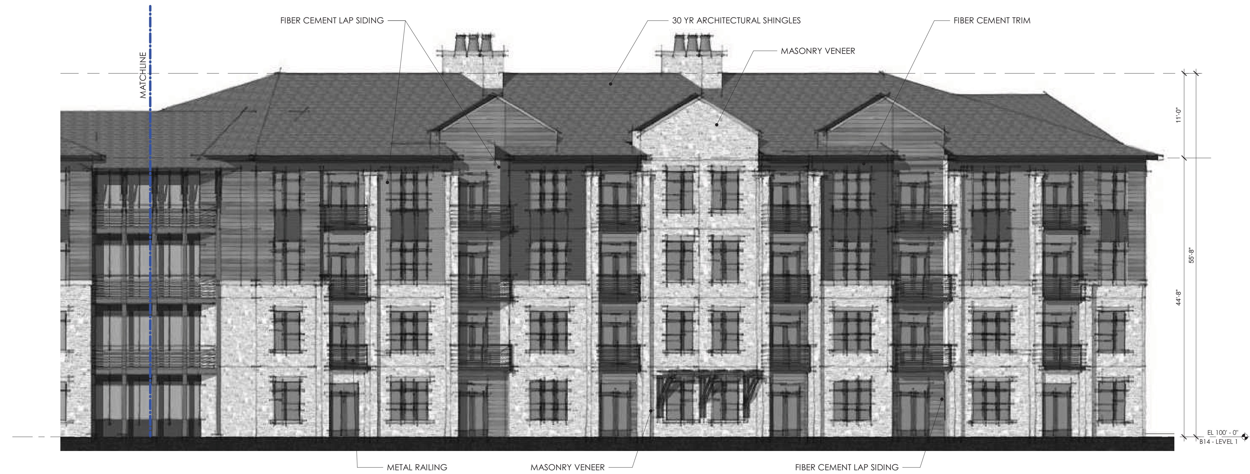
BLDG 14 - 4 STORY RESIDENTIAL - PARTIAL ELEVATION 2
