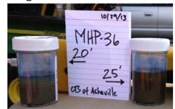
Positive Oil-in-Soil™ test result from soil at 20 and 25 feet below the surface
