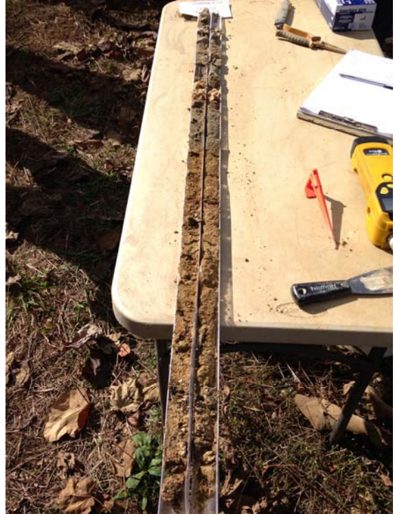
Soil core from 15-20 feet at boring location MHP-36
