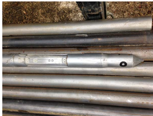
Membrane Interface Hydraulic Profiling Tool (MiHpt)
