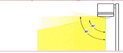
Shield is a device that is attached onto or inserted into a luminaire to alter the direction of light being emitted. A luminaire that has a shield attached or inserted is considered to be "shielded."
