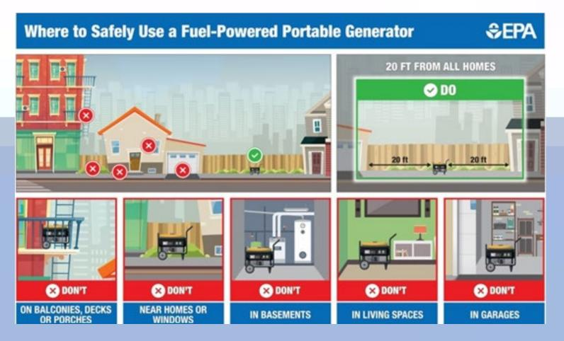
• During power outages, portable generators can be used to help temporarily restore power to a few key appliances like refrigerators, lights and fans. Portable generators that use fuels such as gasoline, natural gas or kerosene are widely available. However, if they are not used correctly they can be hazardous because their exhaust contains deadly fumes, like carbon monoxide. Carbon monoxide is a toxic gas you cannot see or smell but could kill you in minutes.
