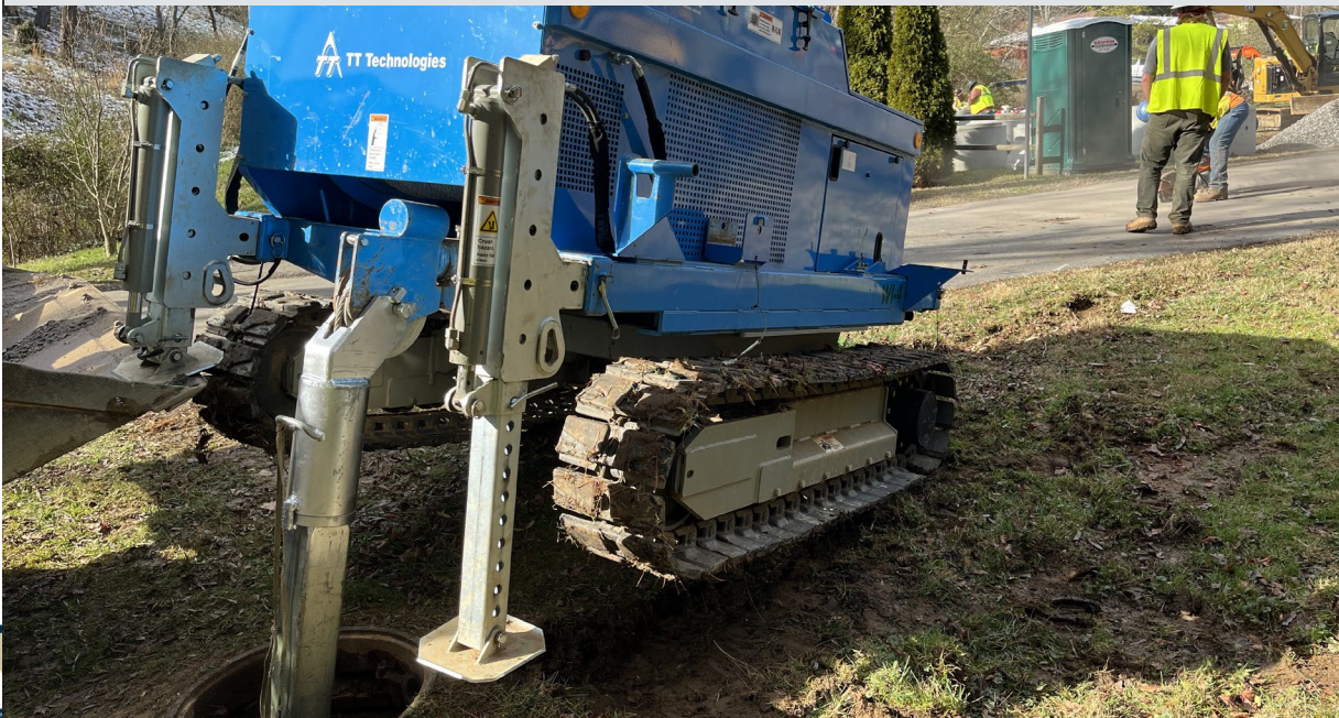
Pipe bursting bore pit (top left); bursting head and HDPE pipe (top right); winch machine (lower left); bursting head entering old manhole (lower right)
