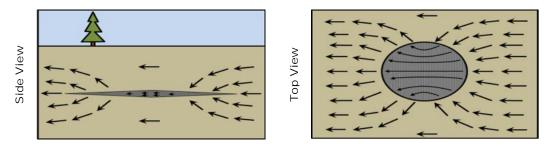
Profile examples of groundwater flow lines converging on a high permeability emplaced structure. (From Hall, et. al., 2013).
