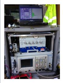
LIF analyzer and computer software readout for a boring in January 2014 (Task 4)
